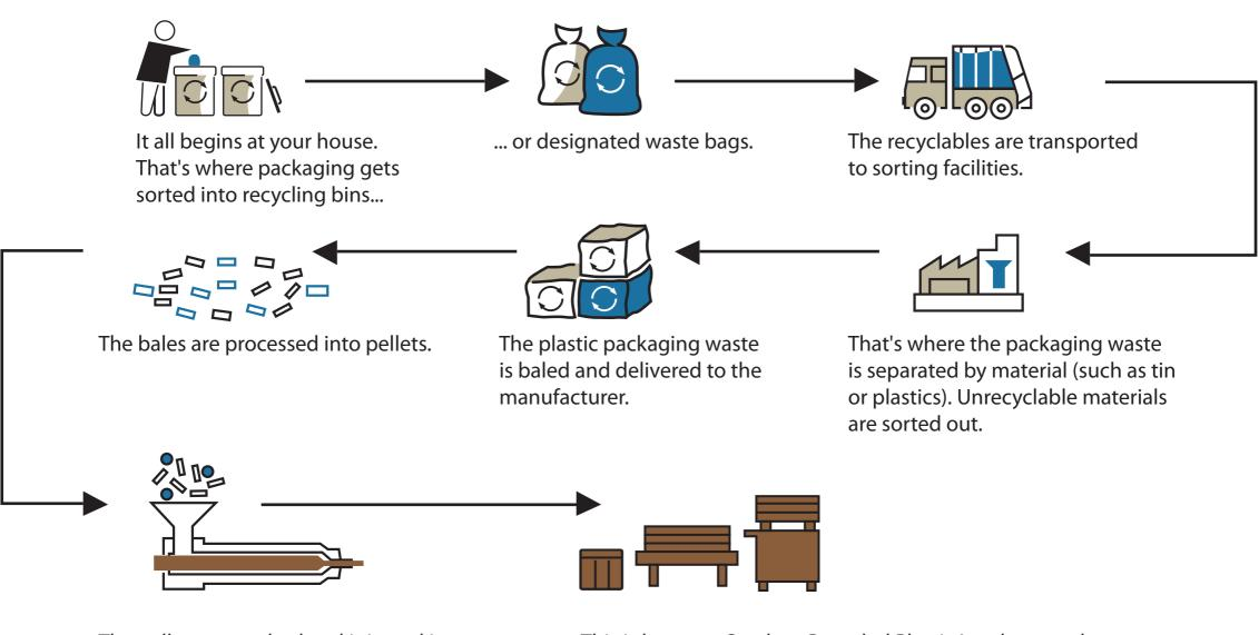
The pellets are melted and injected into molds that are formed into lumber and other shapes. Sometimes color is added at this stage.
